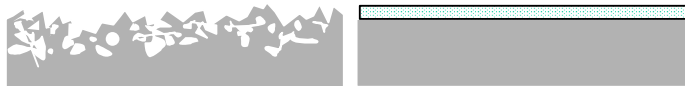
Figure 1 illustrating the idea of an effective medium. The microrough-porous surface on the left can be modelled as a smooth surface with an effective refractive index being some mixture of air and specimen material.
