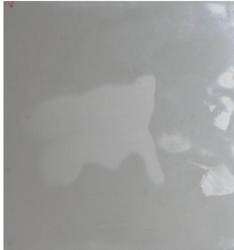
Figure 1b Image of the 20 wt% filled plaque showing significant gate marking features. The gate is at the right centre of the image.
